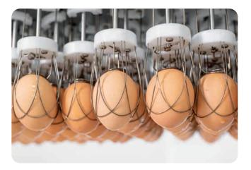
**Haylo™ technology:** On the transfer table and egg remover, Haylo technology removes and transfers eggs with patented loop-wire design, reducing cracks,\*,6 minimizing egg contact and enabling easier disinfection.
