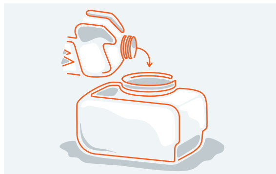
Flush half of a soap solution through the sprayer line and tip.
